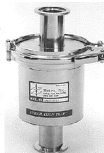
When using a vacuum-filtration assembly, pay strict attention to the liquid levels in the trap bottle. Use a secondary trap bottle so that if liquid in the primary trap bottle reaches the inlet tubes, the liquid will be vacuumed into the secondary container instead of the pump. This will help reduce vapors in the atmosphere and expensive vacuum pump replacement costs.
