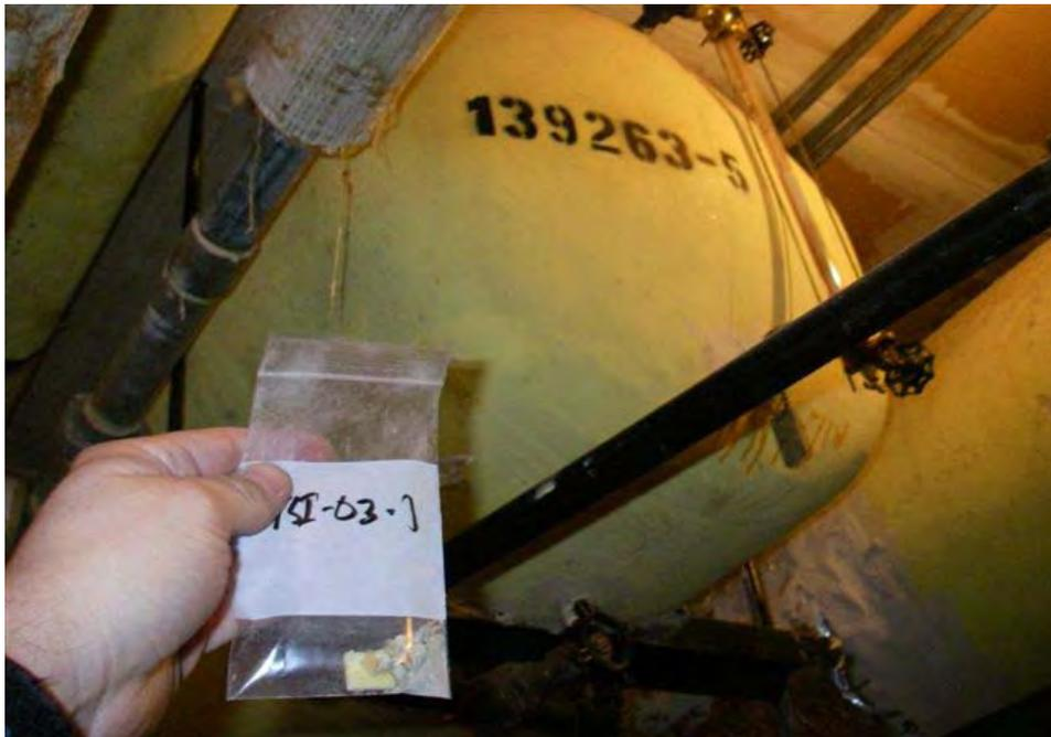
**Sample No. TSI-03-1 to TSI-03-3, Thermal System Insulation (expansion tank insulation).**
