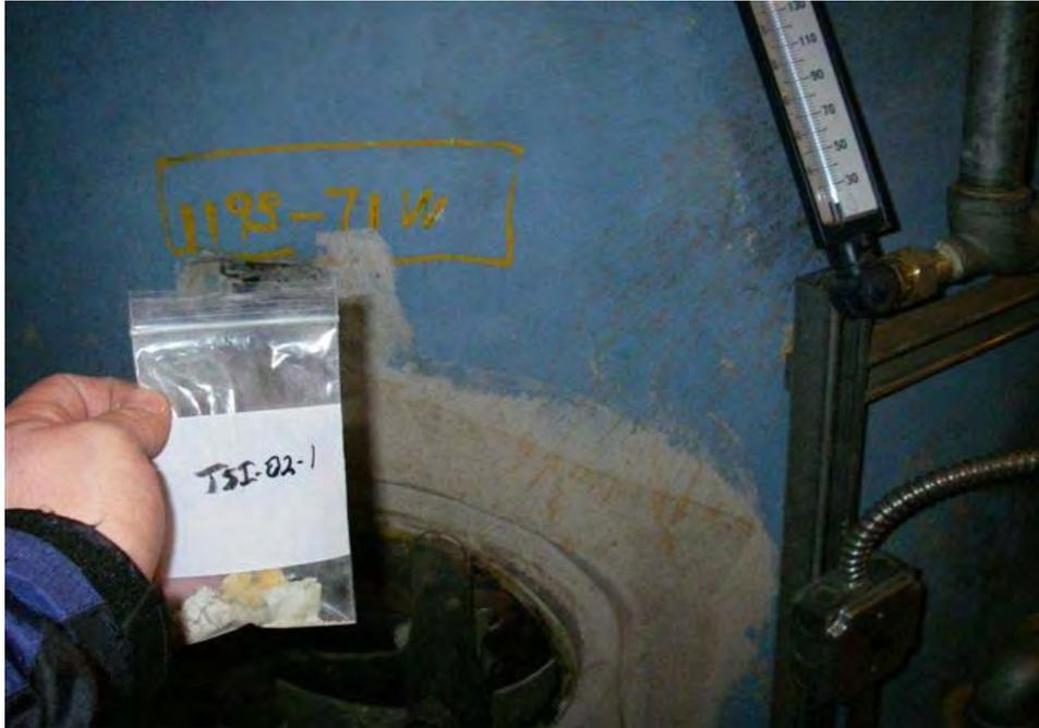
**Sample No. TSI-02-1 to TSI-02-3, Thermal System Insulation (boiler system tank insulation).**
