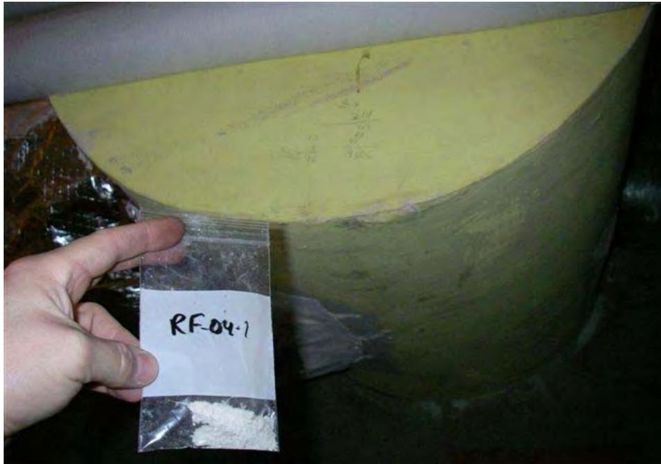
**Sample No. TSI-04-1 to TSI-04-3, Thermal System Insulation (hard mudded fittings on large fiberglass lines).**
