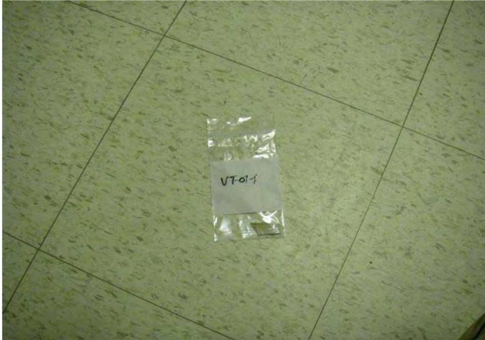
**Sample No. VT-01-1, Asbestos-Containing Vinyl Floor Tile (lt. green 12"x12" with green splotches) with Non Asbestos-Containing Mastic (brown/yellow).**
