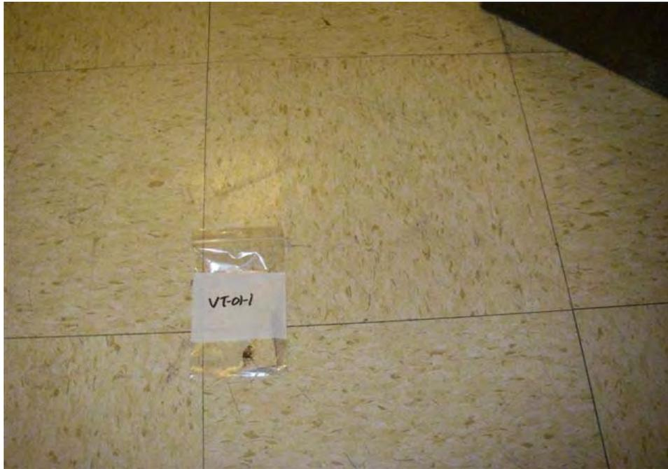
**Sample No. VT-01-1, Vinyl Floor Tile (cream 12"x12" with yellow and green splotches) with non asbestos-containing Mastic (black).**
