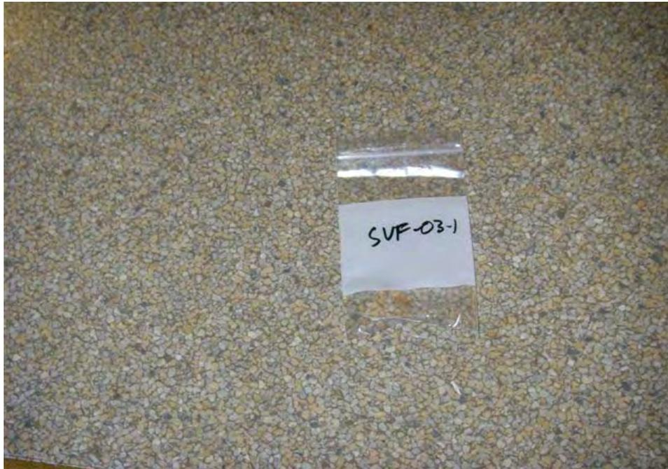
**Sample No. SVF-03-1, Sheet Vinyl Flooring (grey pebble terrazzo pattern) with presumed asbestos-containing Mastic (yellow).**
